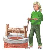
The wheel and axle helps us lift heavy loads, such as a bucket of water, from the bottom of a well.
